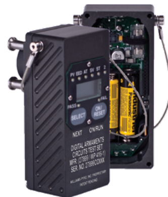
DVD (Digital Voltage Detector) "Juice Box" design replaces the antiquated "Beer Can" tester, with more capabilities
