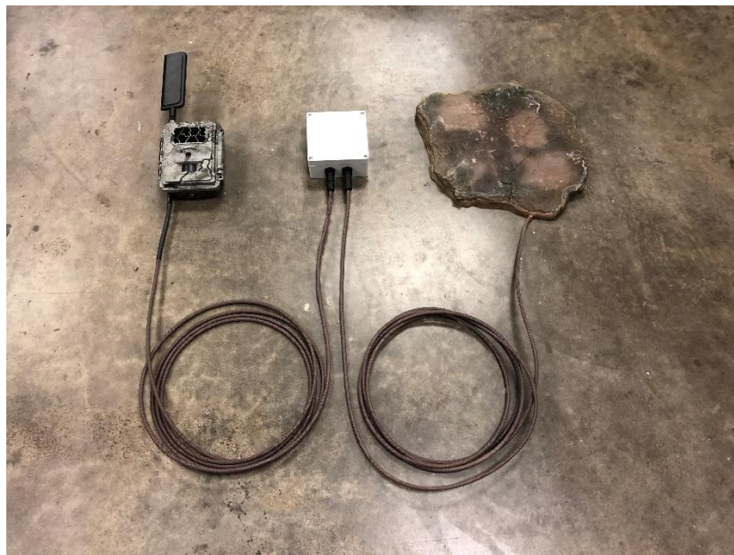
Figure 1: Drawbridge (Spartan) Camera Covert Power System
