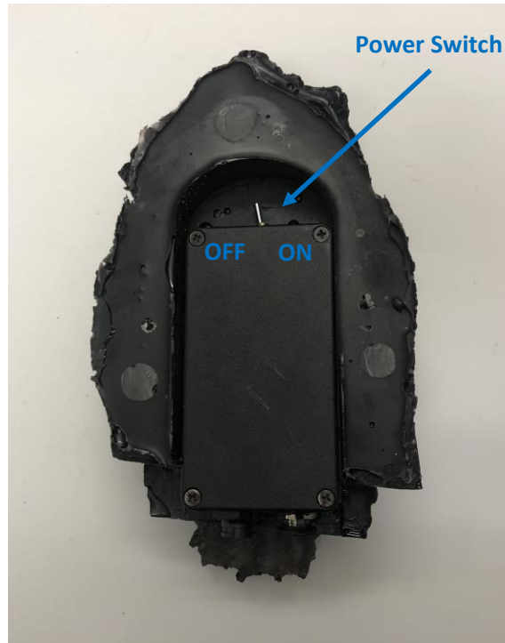
Figure 2: IR Flash Unit Power Switch
