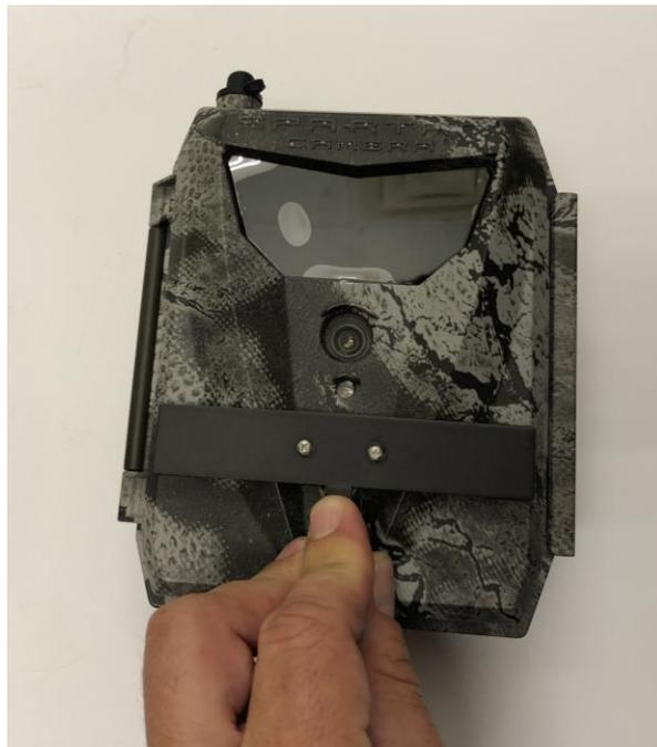
**Figure 18: Attach the Eyepatch Magnets to the Camera Housing**
