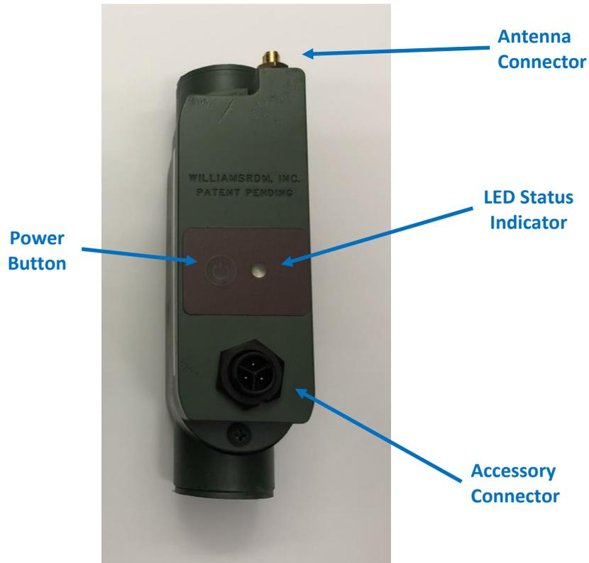
Figure 3: START Sensor Node
