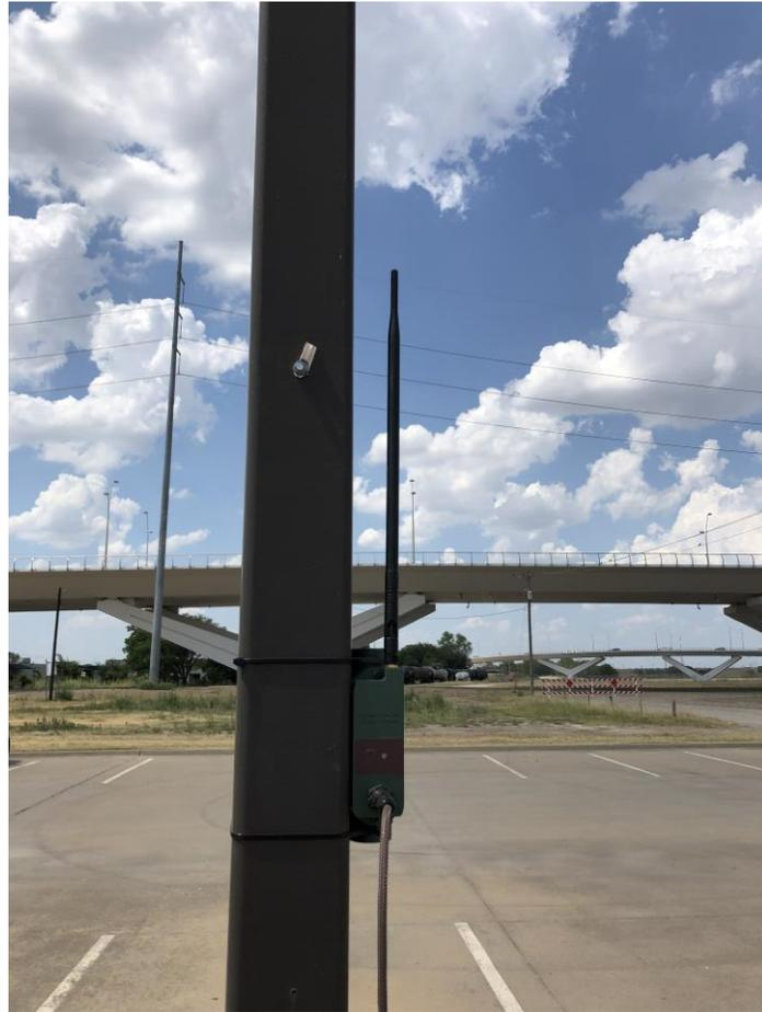
Figure 50: Sensor Node Mounted to a Light Pole
