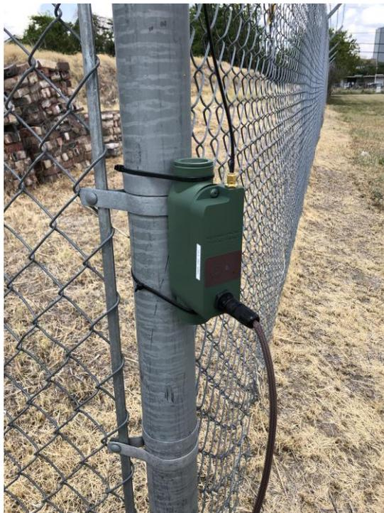
Figure 48: Sensor Node Mounted to a chain link Fence Close Up
