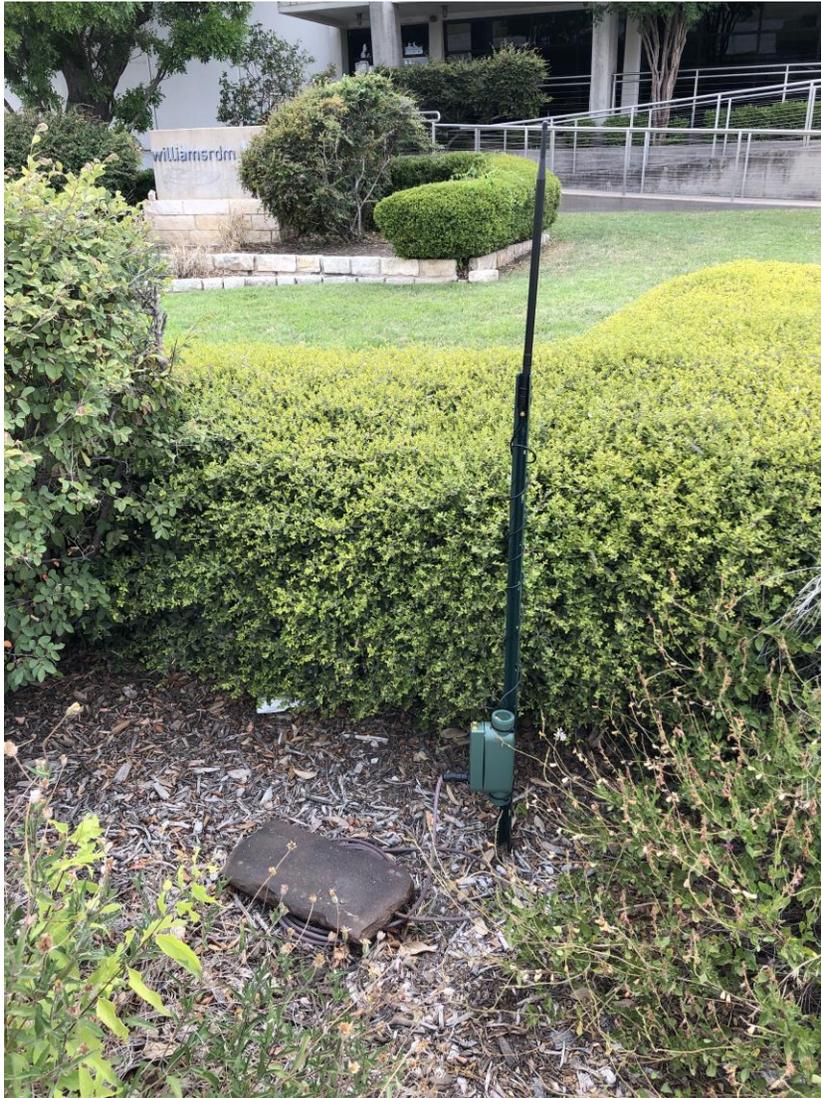
Figure 44: Sensor Node Mounted to a U-Post
