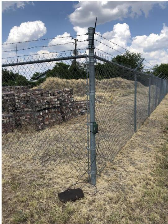
Figure 47: Sensor Node Mounted to a chain link Fence
